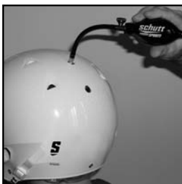
4. Insert Schutt® Model 7790 Inflation Needle with the pump into the valve for the Crown Air Liner which is the top inflation site and should be used when making a crown adjustment. Inflate or deflate the liner through the valve as pictured to insure proper fit. Proper fit should usually require zero to two pumps.
